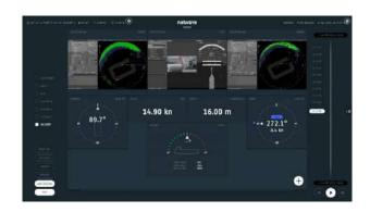
VDRs are data recording systems, mandated for commercial vessels in international waters under regulation 20 of SOLAS Chapter V, to enable accident investigators to review procedures and instructions in the moments before an incident and help to identify the cause of any accident for ocean going vessels.
